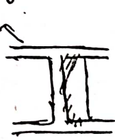
Built up channel section
